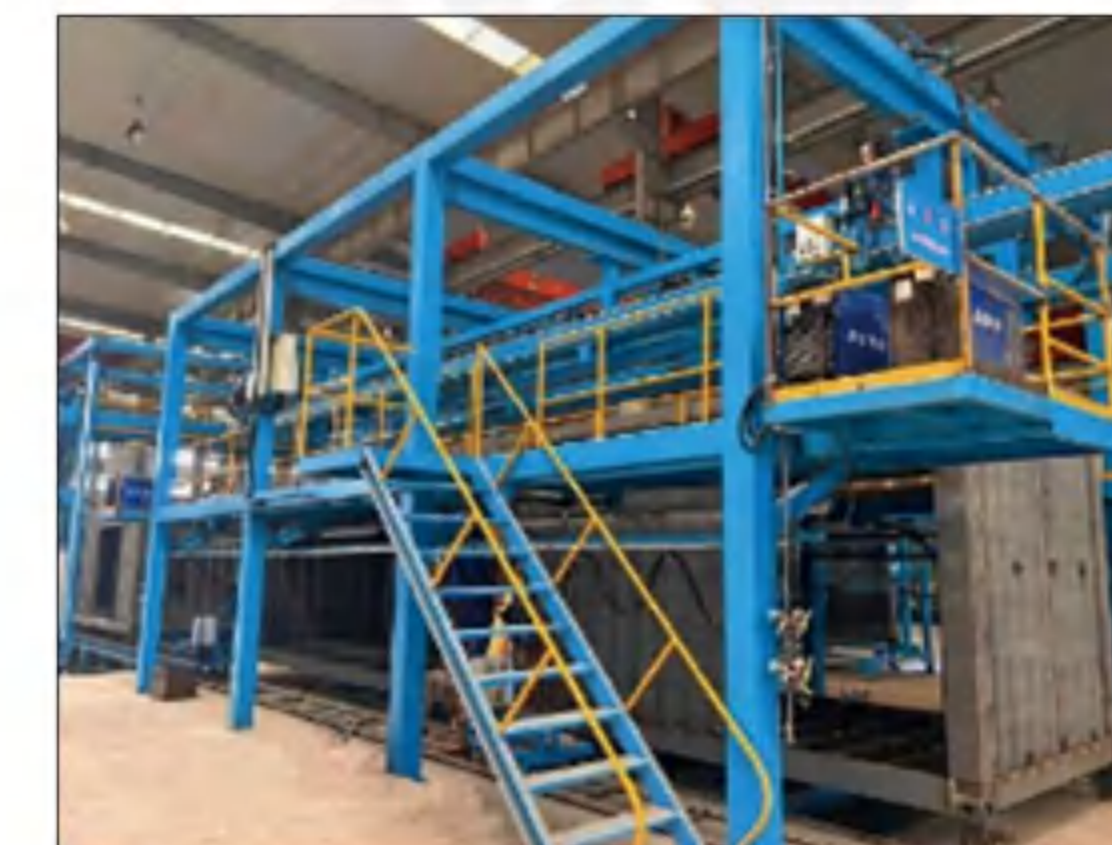
General assembly welding station (18M) 总装焊接站 (18M)
