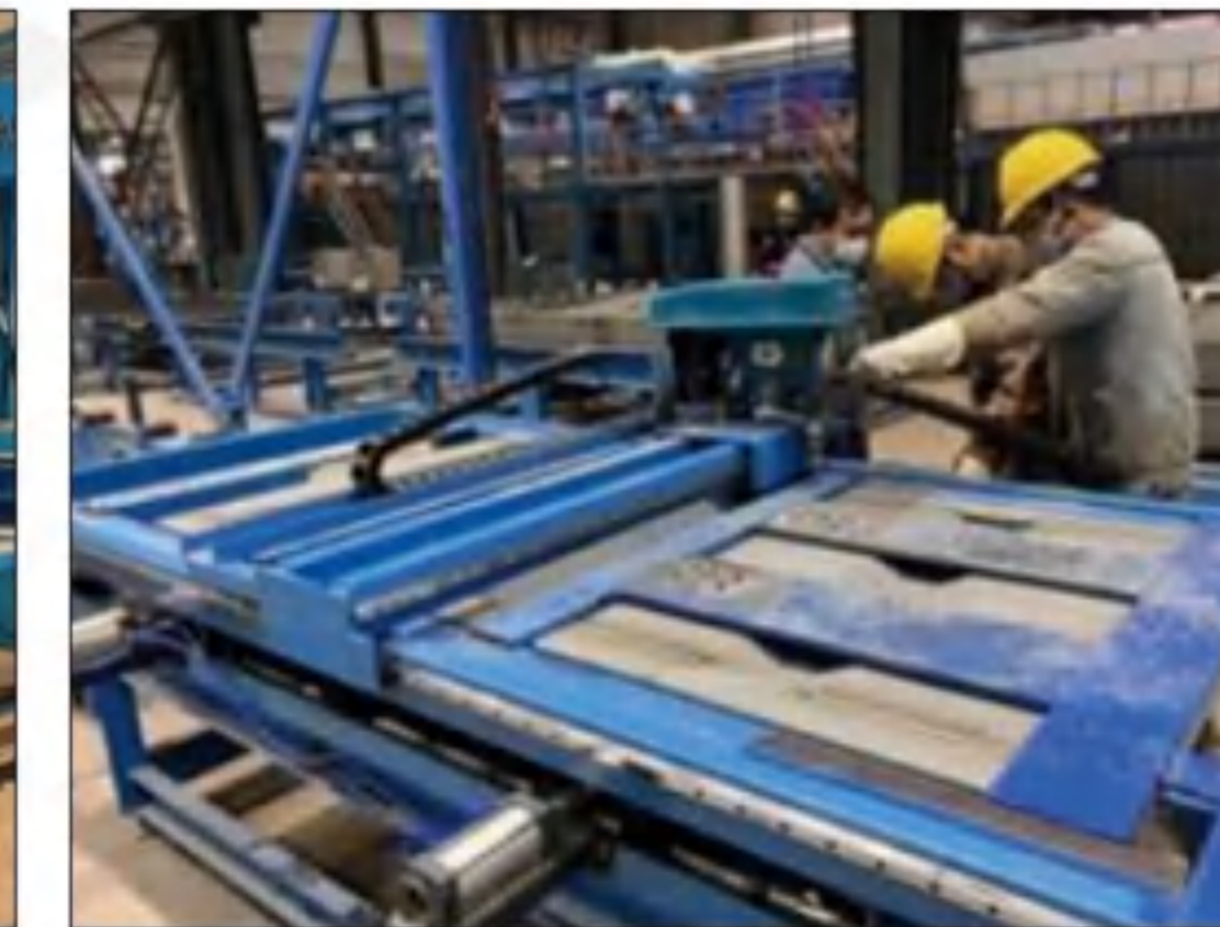
Door holes drilling 门洞钻孔
